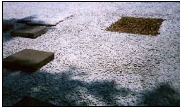
Figure 1. Uncoated patch (upper right) and coated piece (upper left) for solar reflectance samples at Tyndall Air Force Base
